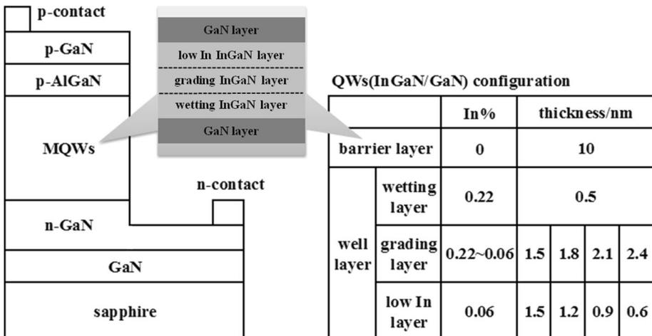
Fig. 1 Schematic diagrams of the redesigned LED
