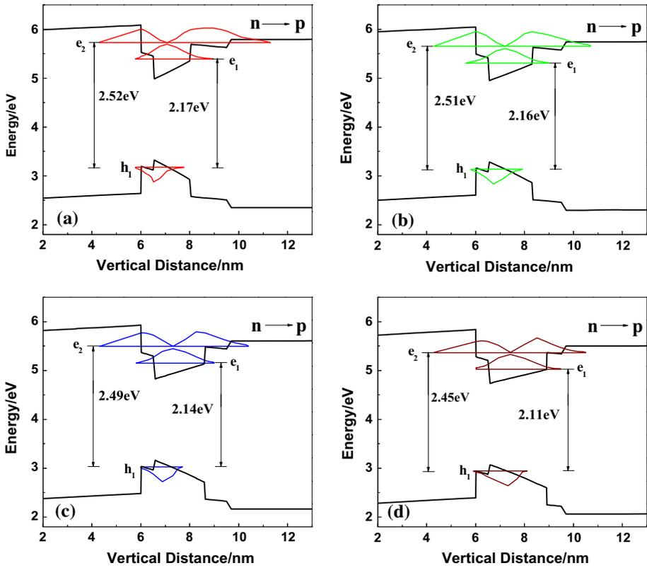
Fig. 3 Energy band diagrams and wave functions of the four QW structures
