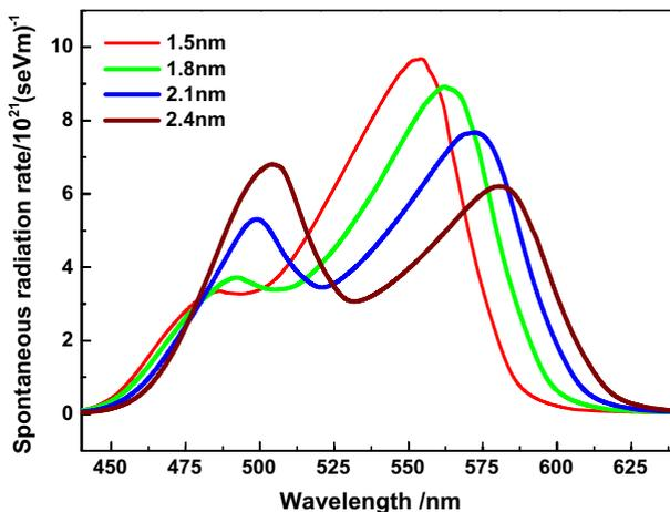
**Fig. 2** Spontaneous emission rates as a function of wavelength for four LEDs
